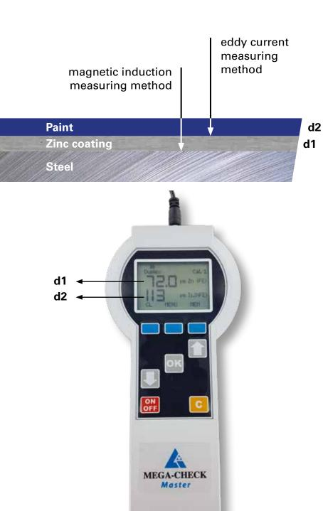
Two measuring techniques are used to measure the thickness of layers over a metal substrate.
