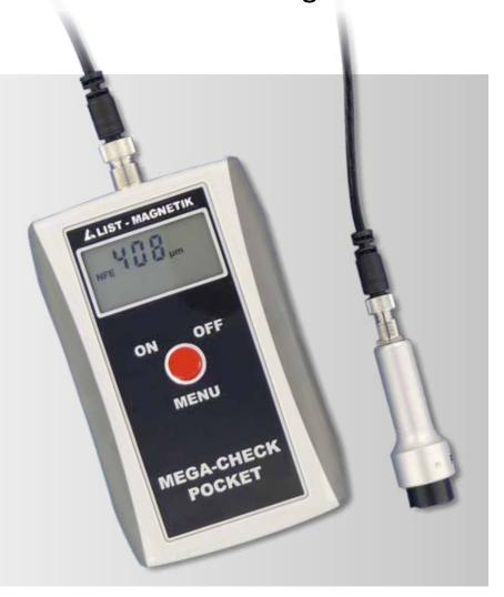
With the LIST MAGNETIK MEGA-CHECK Pocket coating thickness meters, you can carry out exact, reproducible measurements. The measuring probes digitize the signals in the probe before they are transmitted to the measuring device via the probe cable. The probe cable, which can be plugged in on both sides, connects the display unit and probe, and can be easily replaced in the event of a cable defect.
